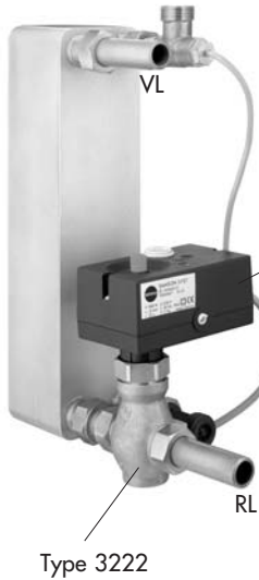
Typical application with Type 3222/5757 Control Valve for domestic hot water heating in instantaneous system
