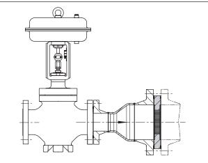
Fig. 5: Type 3381-1R: Reduced construction downstream of the pipe expander
