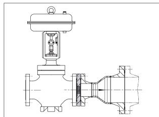
Fig. 3: Type 3381-1: Attenuation plate at the valve upstream of a pipe expander
