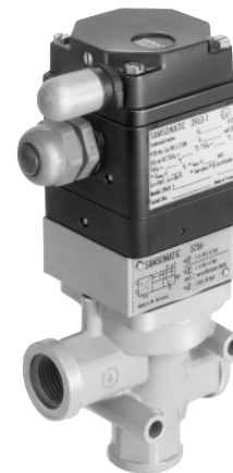
3/2-way solenoid valve, single actuated with spring return mechanism, K_{vs} 4.3, connection G 1/4
