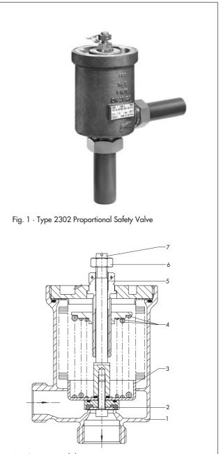
Fig. 2 · Functional diagram
